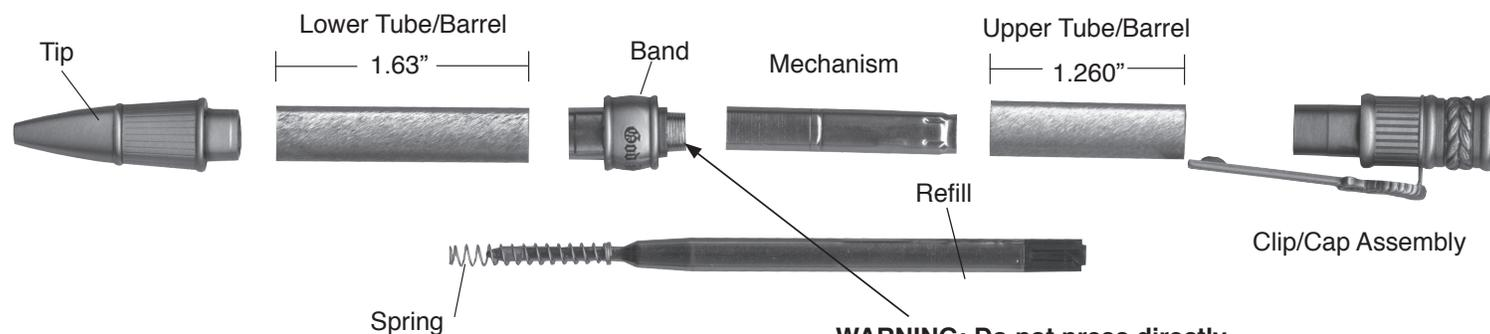
**WARNING: Do not press directly againsts these threads. Use a pressing block. See Assembly Instruction**
